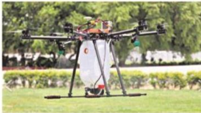
Drone sanitiser designed and developed by the students of Lords Institute.
